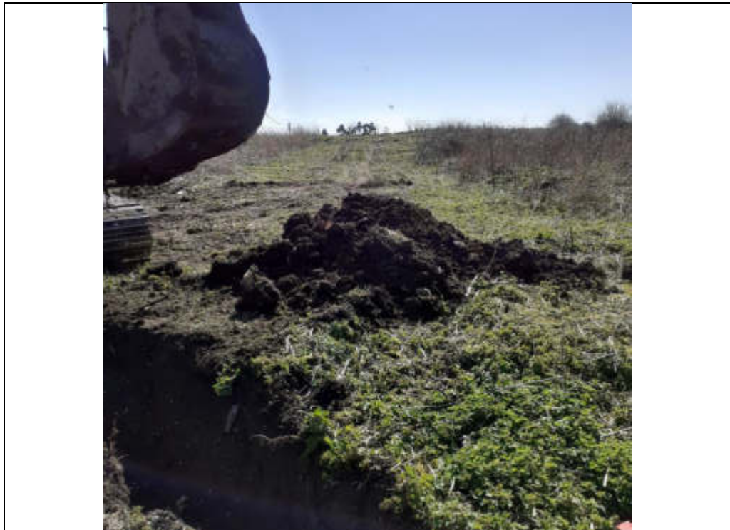
Plate 241: TP128 ranging from ground level to 1.6 m bgl.
