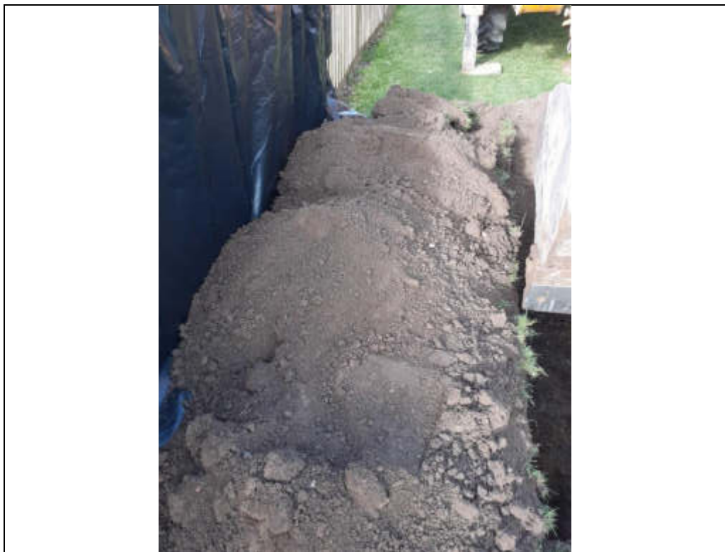
Plate 18: TP103 ranging from ground level to 0.8 m bgl.
